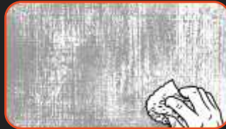
phase VI: Using a sponge, apply Decorative Varnish coloured with 20 ml pigment, two separate colours, in such a way that they blend into each other.
