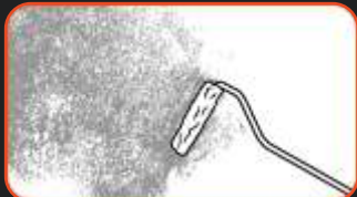
phase I: Apply Decorative Concrete with a roller upon the surface previously primed with the Bonding Primer.
