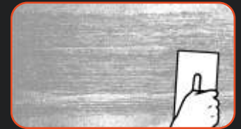
phase III: Model the pattern by dragging a brush trowel over the plaster.
