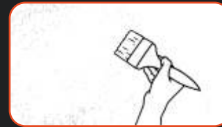
phase I: Coat the clean and dry surface with the Bonding Primer.
