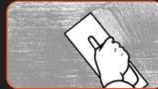
phase IV: When the surface is dry, apply another layer of the material.
