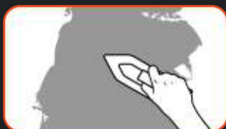
phase II: Apply layer of Pearl Relief with irregular moves of a plastic trowel in order to form the pattern.
