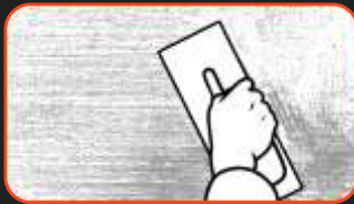
phase II: Apply Sandstone using a Venetian trowel.
