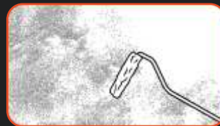
phase III: When the first coat dries, apply the second coat of Diamento similarly to the previous one.
