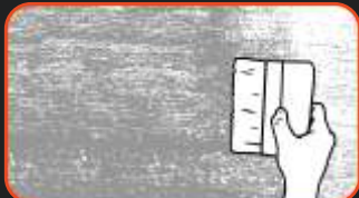
phase IV: Cover surface with the colourless Decorative Varnish.
