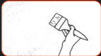
phase I: Apply the Bonding Primer upon clean and dry surface.
