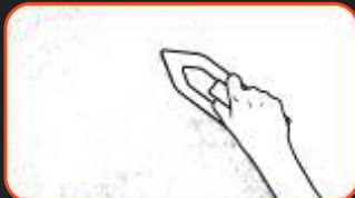
phase II: Smoothen the surface with a plastic trowel.
